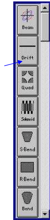
Individual optics elements (PBO Lab Pieces) are located on the scrolling Palette Bar of the OModule Specification Document.
